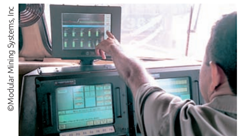
©Modular Mining Systems, Inc A Vale engineer uses the SmarTrain on-board computer
