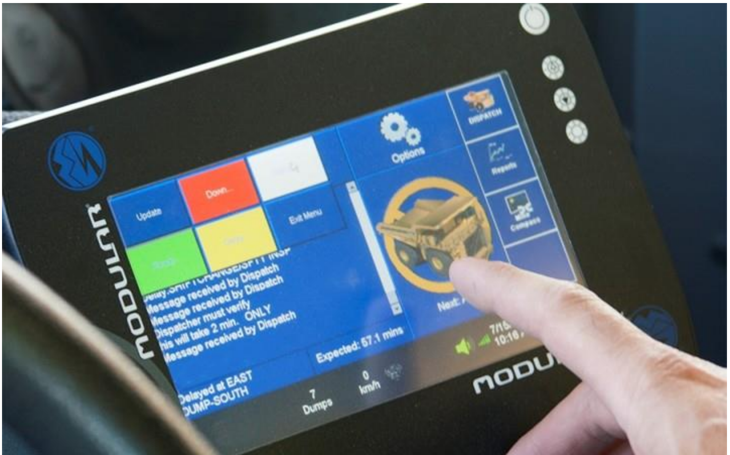
Modular Mining Systems' DISPATCH fleet management system will optimise haulage operations on Pico's fleet
