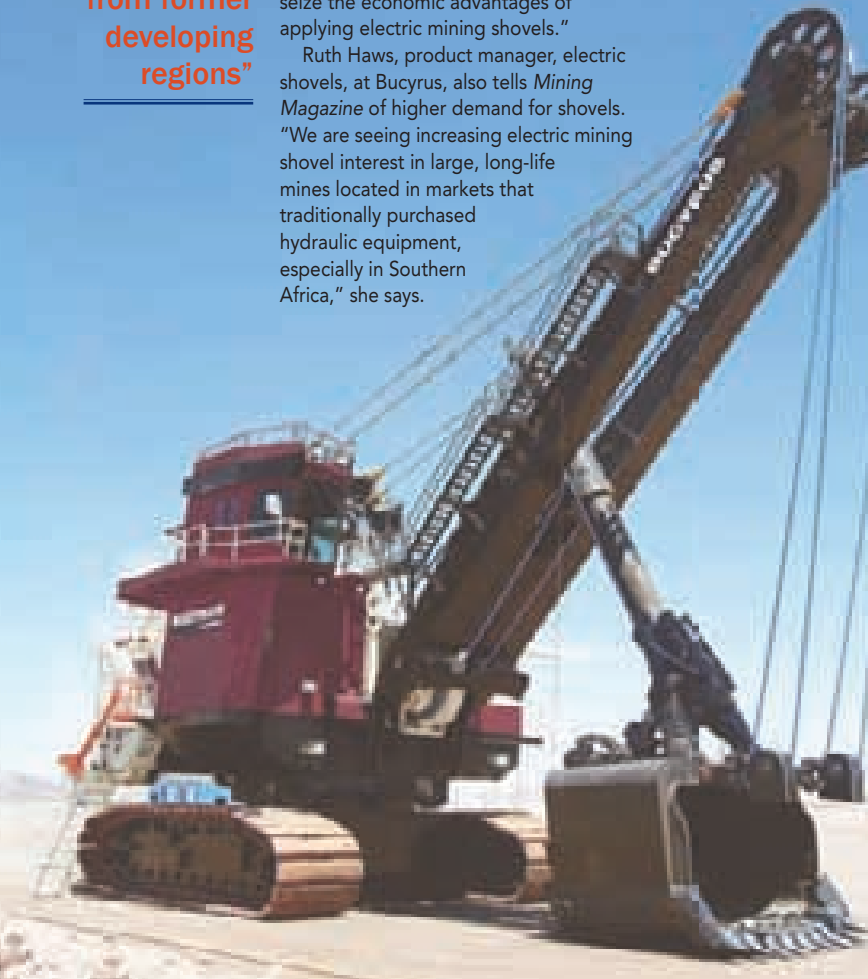
Bucyrus 495 HR2 electric rope shovel
