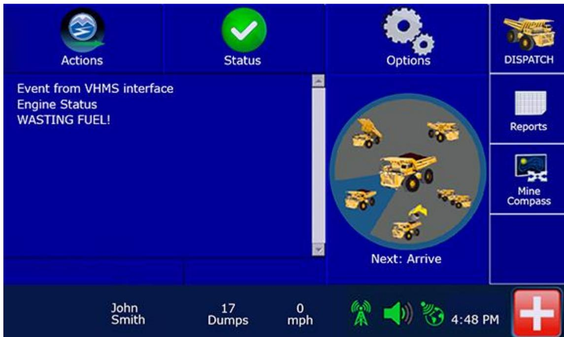
As a long-time user of Modular's DISPATCH® fleet management system, the mine turned to Modular to help them identify and manage the occurrence of idle events and reduce rising fuel costs. Modular worked with mine personnel to conceptualise and develop a solution to help increase awareness of wasted fuel: the DISPATCH idle monitor module.
