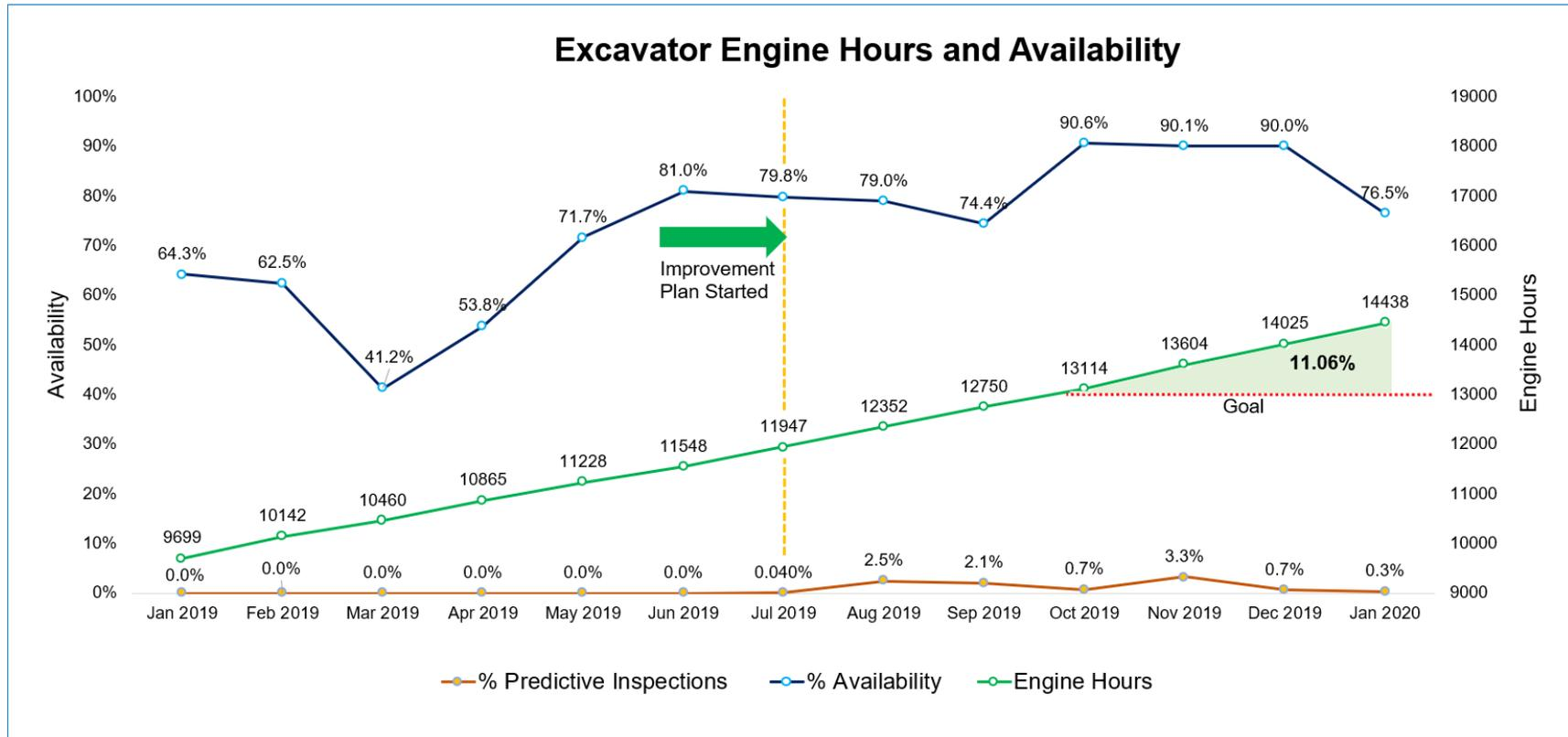
Figure 1. By the end of the MineCare team's improvement plan, the excavator engine's runtime and availability increased by 11% and 11.6%, respectively.
